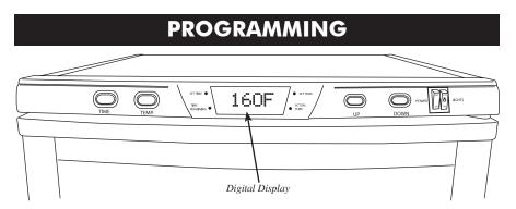
7. **TO SET THE TIME**: Press the **"TIME" Button** on the **Control Panel** one time. Use the **"UP"** & **"DOWN" Buttons** on the right side of the **Control Panel** to set the countdown timer hours (23 hour maximum). Press the **"TIME" Button** again to switch to minutes. Similarly set the minutes (5 minute increments).
